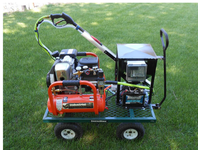
Fig. 1. Portable abrasive grit applicator showing the air compressor, grit tank, battery-powered auger, air and grit hoses, and trigger-operated single-nozzle wand. [Colour online.]
