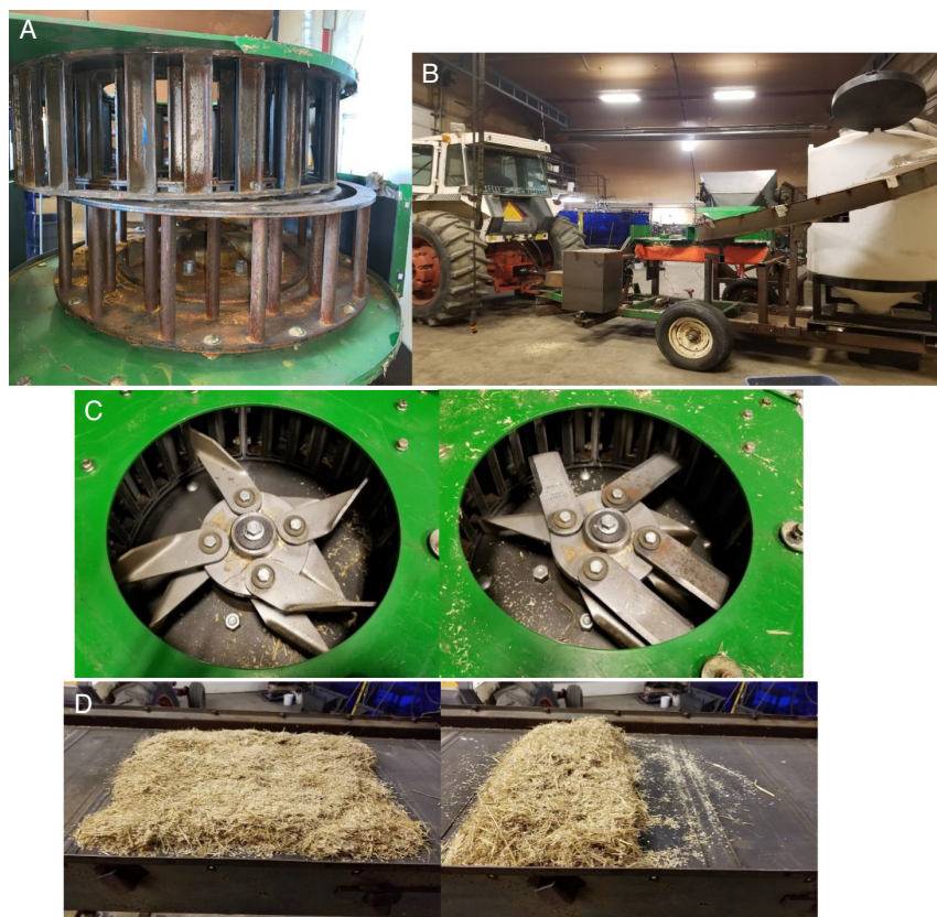
Fig. 1. (A) The Redekop Seed Control Unit™ (SCU) disassembled so that the blade system is visible in the center of the rotor plate (bottom). (B) The SCU set up for stationary testing. (C) The eight fan blade system treatment (left) and the four cutting blade plus four fan blade system (right). (D) The 5 Mg h -1 (left) treatment and the 10 Mg h -1 treatment (right). [Colour online.]
