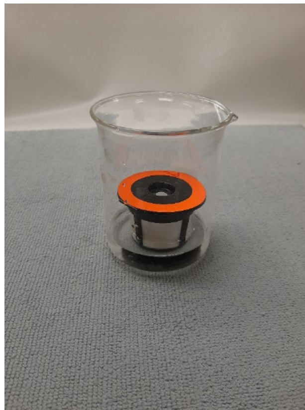
Fig. 4. Experimental setup used to estimate zeolite and NaOH-treated phosphorylated wood pulp fibers affinity for calcium ions.
