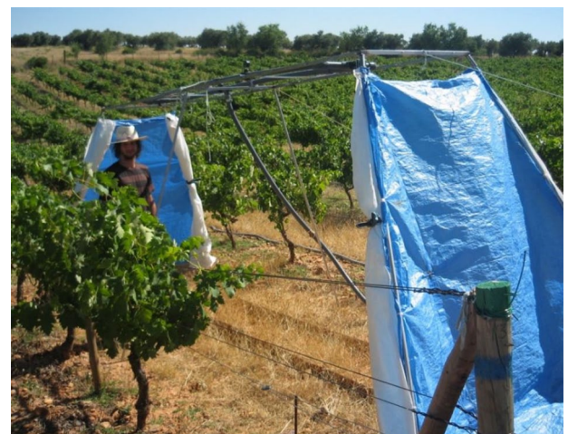
Figure 2. Rainfall simulator. Two full cone nozzles placed in an operating height of 2 m above ground. The windbreaks are partially placed around the simulator in the picture. During the experiment, the windbreaks were unfold completely for preserving rainfall distribution.
