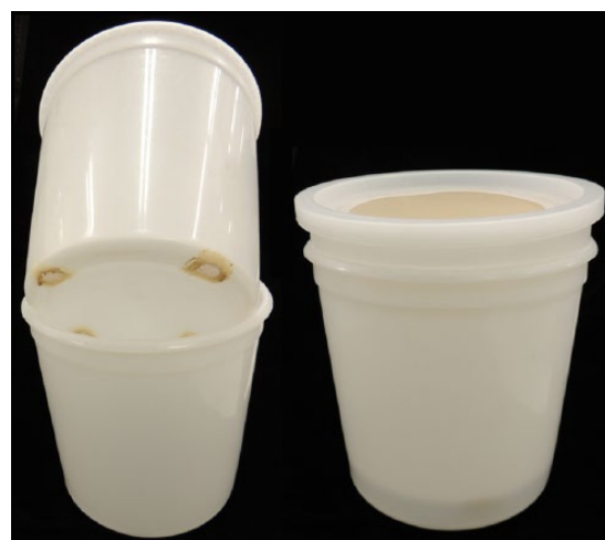
Figure 3. Plastic buckets used for holding fruits for assessment of infestation by tephritid fruit flies. The picture on the left shows the screened bottom holes on the top bucket that permitted the draining of fluids from the fruit to prevent drowning of any infesting tephritid fruit fly larvae. The picture on the right shows the screen on the lid of the top bucket and the buckets as stacked together. Photo by G.T.M.
