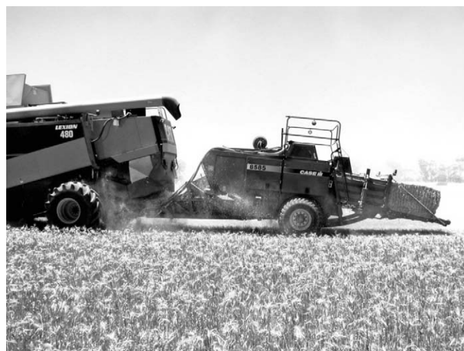
Figure 3. Bale direct system collecting and baling chaff and straw residues during wheat harvest.
