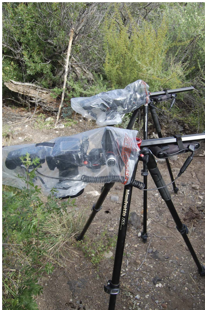
Figure 2.—Camera set-up over nests of Novomessor albisetosus ; field of view includes main nest entrances as well as an extensive area surrounding the nest entrance (approximately 0.152 m 2 covered by each camera).
