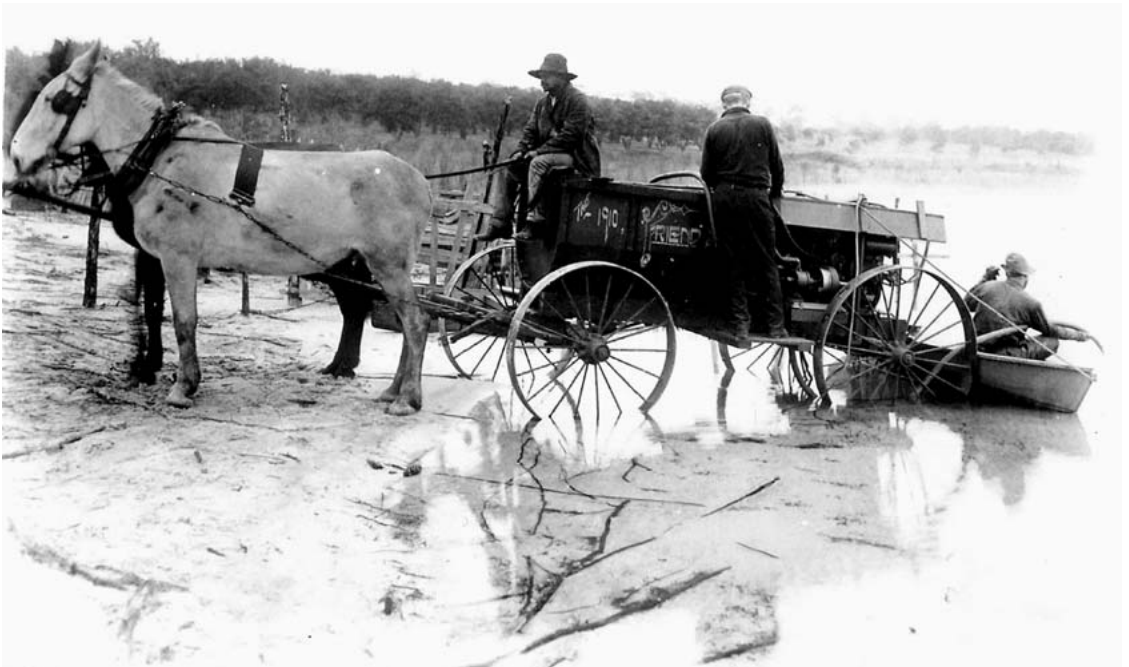
Fig. 7. Horse-drawn spray rig for spraying orange trees with experimental insecticides used by W. W. Yothers, about 1910. Yothers, in the boat at the right of the picture, is seen with a suction hose for obtaining water from the lake to fill the spray tank.
