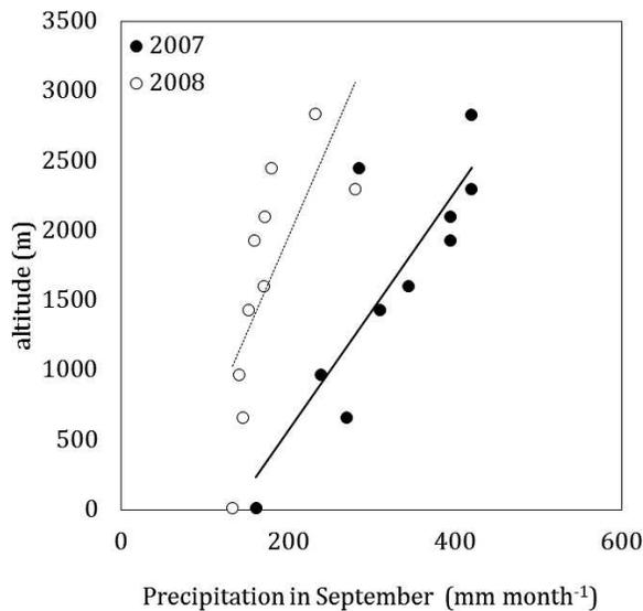
**FIGURE 7.** The relationship between rainfall and altitude in 2007 and 2008. ● and the dotted line represent September 2007 ( $R^2 = 0.52$ ,  $y = 13.86x - 821.8$ ). ○ and the solid line represent September 2008 ( $R^2 = 0.71$ ,  $y = 8.57x - 1146.8$ ). Except for Jodo-daira, the rainfall data are from Honoki and Watanabe (2008) and Honoki et al. (2009).
