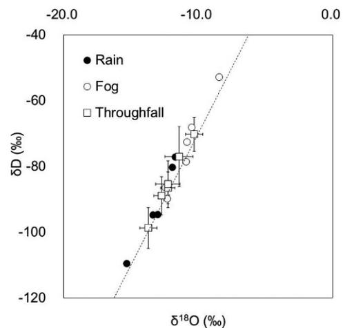
FIGURE 6. The relationships between  $\delta\text{D}$  and  $\delta^{18}\text{O}$  of rainfall (●), throughfall (□), and fog (○) deposition for summer (July–September) at Jodo-daira in 2007 and 2008. Each point shows the precipitation-weighted average value of a month. Error bars show the standard deviation of six throughfall collectors in each month. The dotted line shows the global meteoric water line ( $\delta\text{D} = 8 \times \delta^{18}\text{O} + 10$ ; Craig, 1961).
