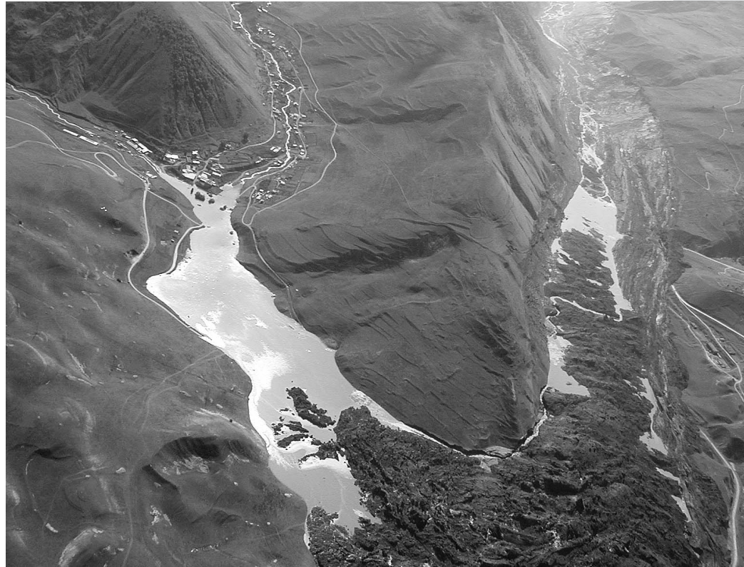
FIGURE 4 View of the mass blocked by the Skalistyi Ridge, and of the rising lake near Saniba. (Photo by Geological Survey of North Ossetia)
