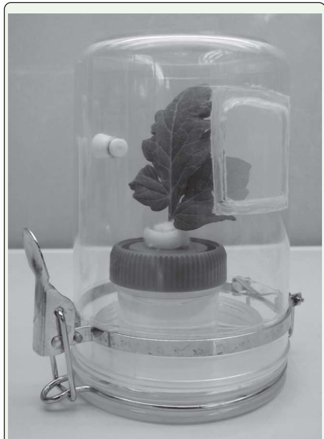
Figure 1. A clear plastic cell containing whitefly nymphs on a water-cultured tomato leaf used for the evaluation of host feeding and parasitism by whitefly parasitoids, Encarsia formosa .
