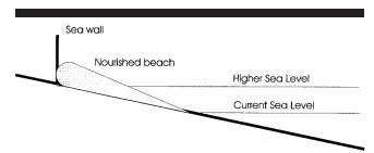
Figure 1. Schematic diagram of response to higher sea level, including a sea wall and a nourished beach.
