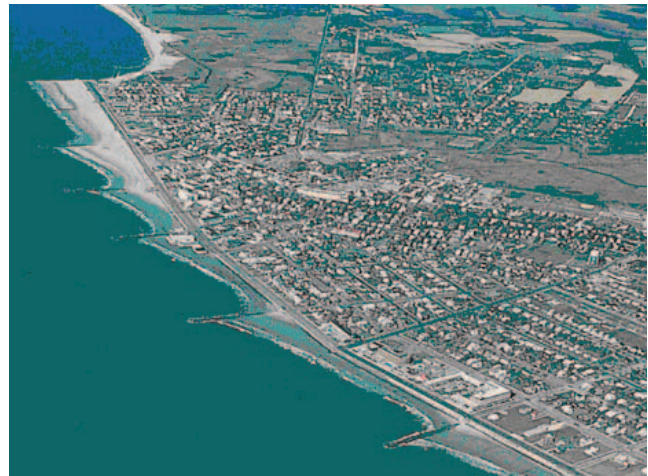
Figure 3. Aerial photograph of New Jersey shoreline showing eroded, cuspate shoreline downstream of groins. (Color for this figure is only available in the online version of this paper.)
