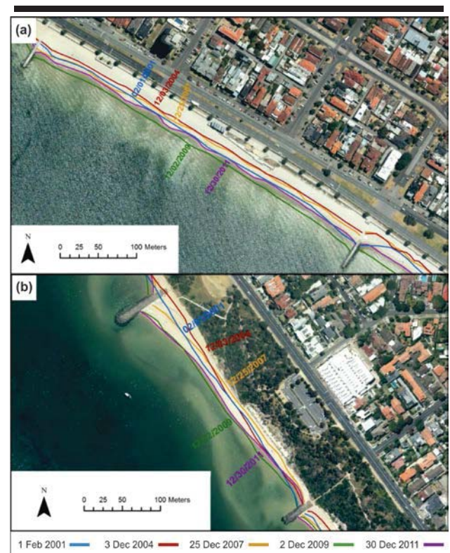
Figure 4. (a) Shoreline change at Middle Park between 2001 and 2011, showing shoreline accretion due to renourishment in 2009 (green line), followed by subsequent erosion (pink line). (b) Shoreline orientation at Sandringham as influenced by the construction of the northern groyne in 2006; the blue and red lines show the pre-groyne shoreline orientation. This area was also renourished in 2009.
