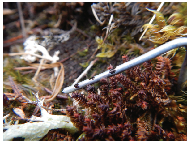
Figure A2. Illustration of the cranked wire method. The picture is from the beginning of the growing season. The tip of the shoots that were measured were aligned with horizontal part of the wire, and the position along the shoot indicated by a black mark on the wire to avoid measuring the wrong shoots at the end of the growing season. Identifying the shoots that were measured was the main challenge with this method (Photo: K. Wangen).
