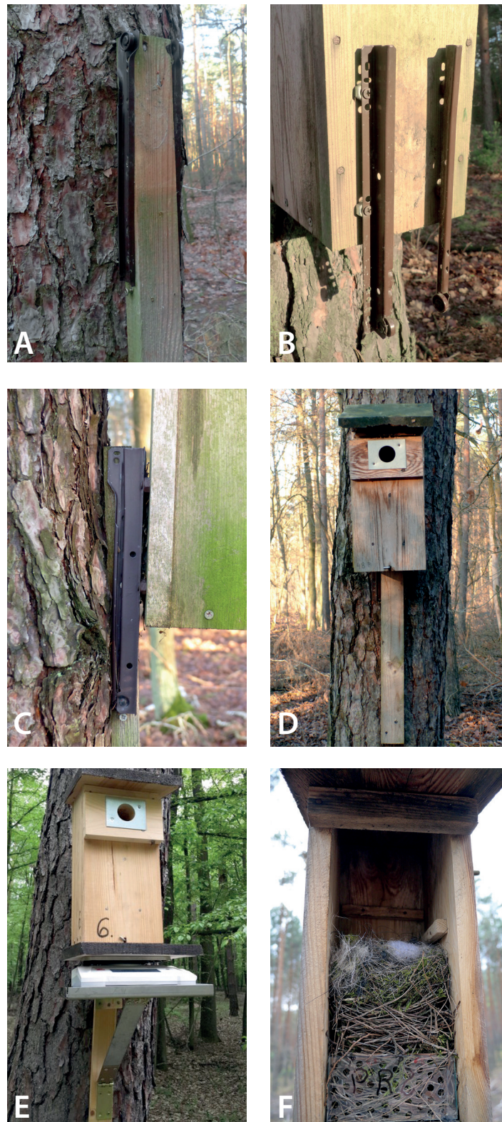
Fig. 1. Modified nest box. A – roller slides attached to the top of wooden mounting strip, B – roller slides attached to the rear wall of the nest box, C – nest box placed stable in the slides, D – nest box mounting strip is long enough to mount a base for the scale, E – a set ready for measurements: nest box with a height pad on the scale, note the base for the scale with a bracket mounted to the strip, F – great tit nest built in a plastic liner.
