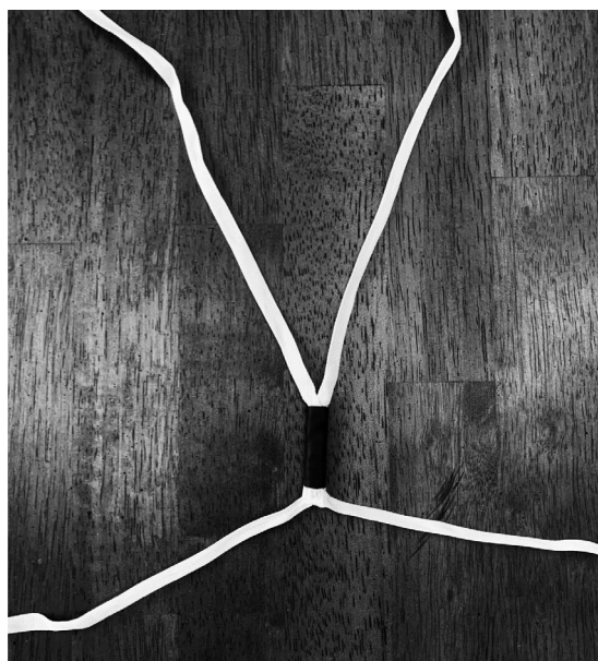
Figure 1. The Y-transmitter Spectra harness attachment design with a reinforced sternum-connecting-ribbon consisting of one additional piece of Spectra and a piece of flexible plastic cutting board mat, covered by heat shrink tubing
