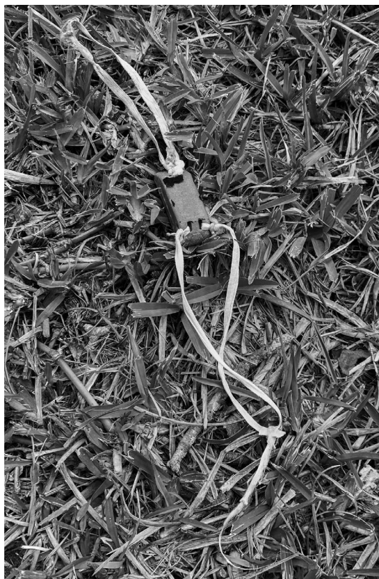
Figure 5. OrniTrack-10 GPS-GSM transmitter with what remained of the Y-transmitter Spectra harness, recovered from an adult female Gray Hawk. She removed the harness by biting through the sternum-connecting-ribbon in <27 d.
