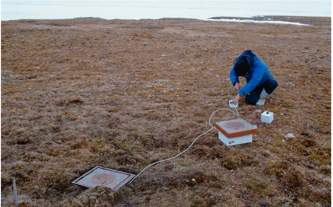
Figure 2. Body mass of Brent Goose females was determined by battery powered balances which were placed beneath nests. One weighing platform has been dug in the ground and is ready for the nest with eggs to be placed on top of it (left foreground). To the right a complete balance is visible. Cables connect each balance with a central computer in a nearby observation hut (photo Jan van de Kam).
