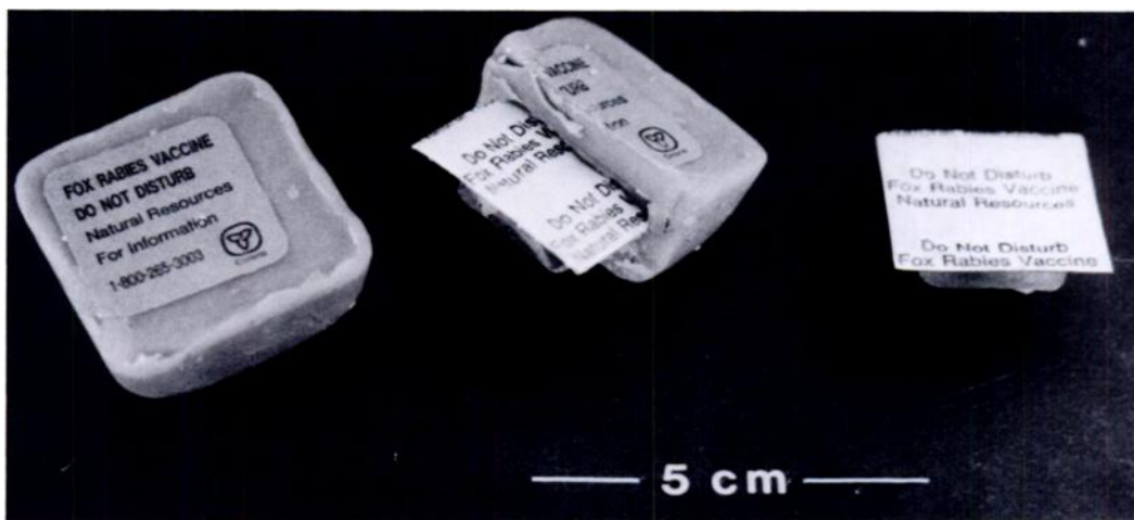
FIGURE 2. In 1987 the blister pack (BP) bait was a labelled cube (left) consisting of tallow, mineral oil, wax strengthener, commercial chicken essence, green food color and tetracycline. The rabies vaccine (2 ml) was carried in a BP placed in the center of the cube (center). The BP was a polystyrene container with a labelled plastic and aluminum foil cover (right).
