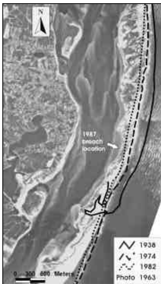
Figure 2. Shoreline changes of Nauset Spit from 1938 to 1982 as determined from vertical aerial photographs. Note that the amount of shoreline recession during this period increased in a southerly direction along the spit.
