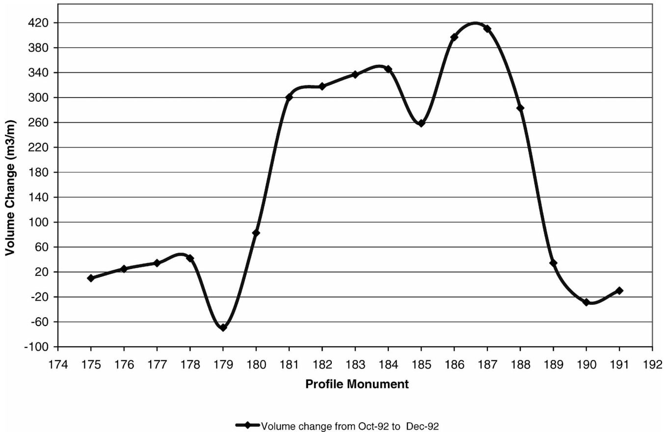
Figure 8. Volume changes from October 1992 (preconstruction survey) to December 1992 (postconstruction survey) showing distribution of fill sands. The nourishment is delimited between monument profiles R180 to R188; higher volumes were placed in the south end of the fill (profile monuments R186 and R187) to counteract higher erosion rates observed in this area after the previous fills.
