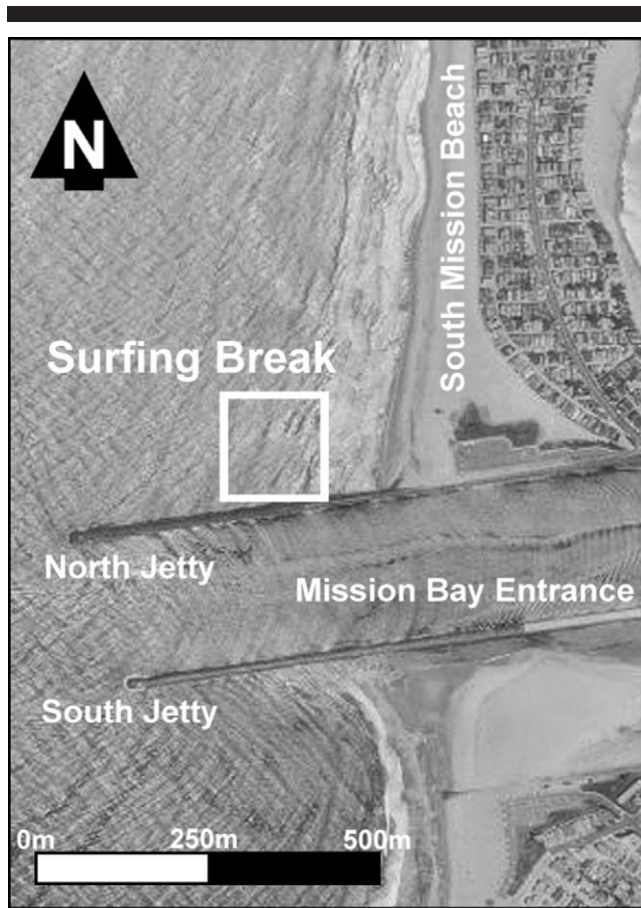
Figure 8. Aerial photograph of Mission Bay jetties, and location of the surfing break created by the northern jetty wall.
