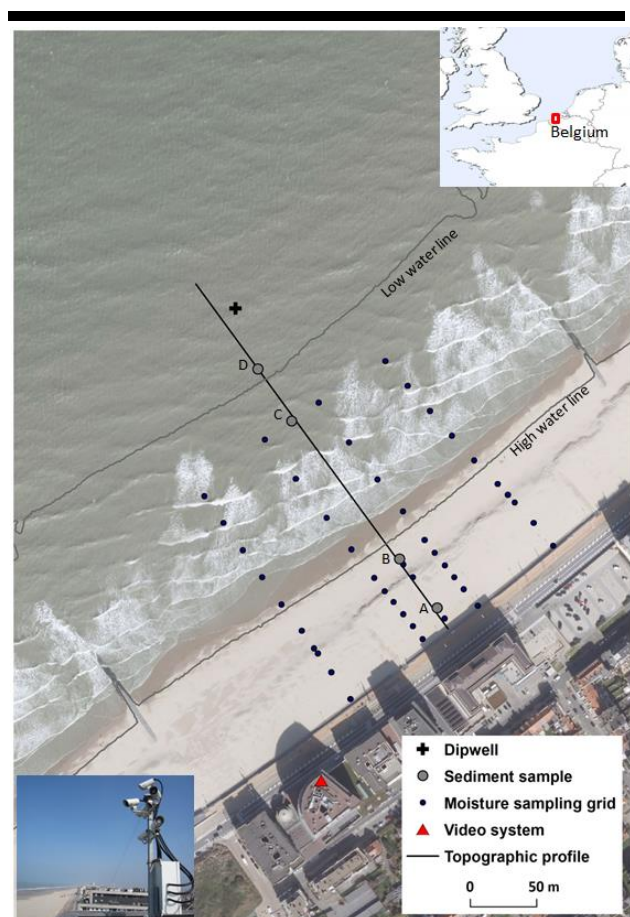
Figure 1. Field deployment and surface moisture sampling grid. Insets: location of the study site and set-up of the Argus video system at the study site.
