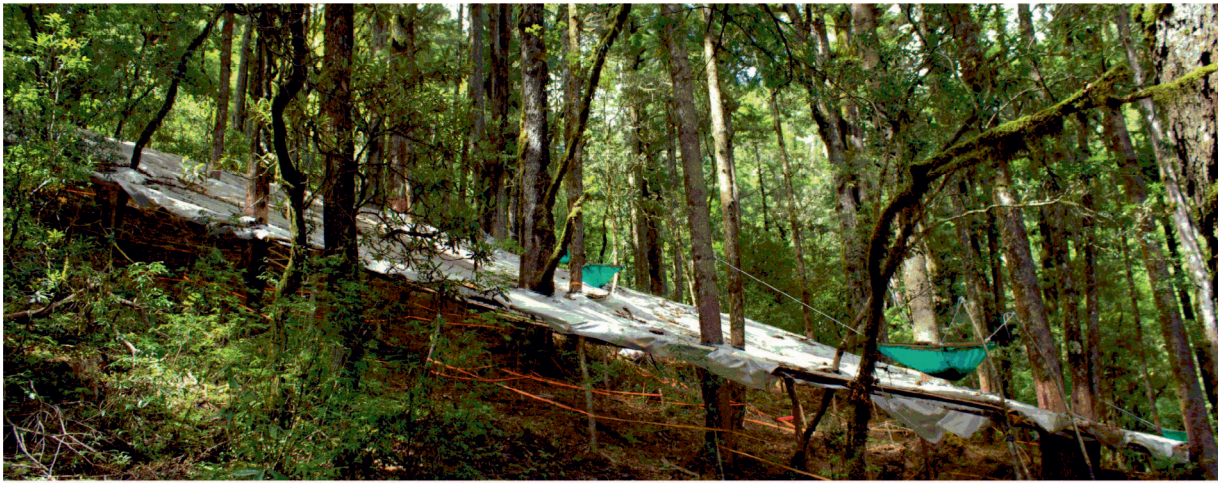
FIGURE 5 Experimental manipulation of precipitation using temporary plastic roofs (top) resting on 1–1.5 m bamboo poles (middle). Upslope of the roofed plot, a trench (bottom) was dug to prevent interflow of water.
