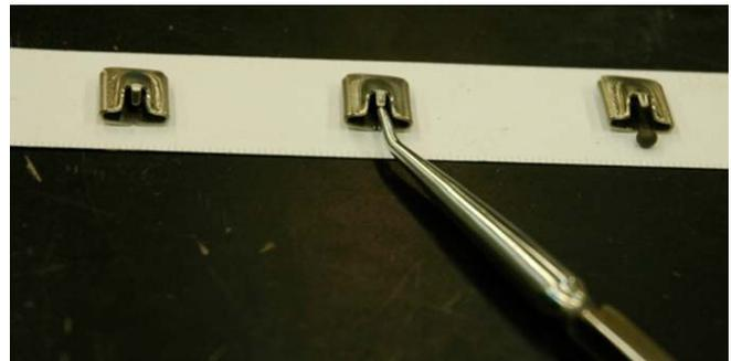
Fig. A1. Preparation of dendrometer band collar.
