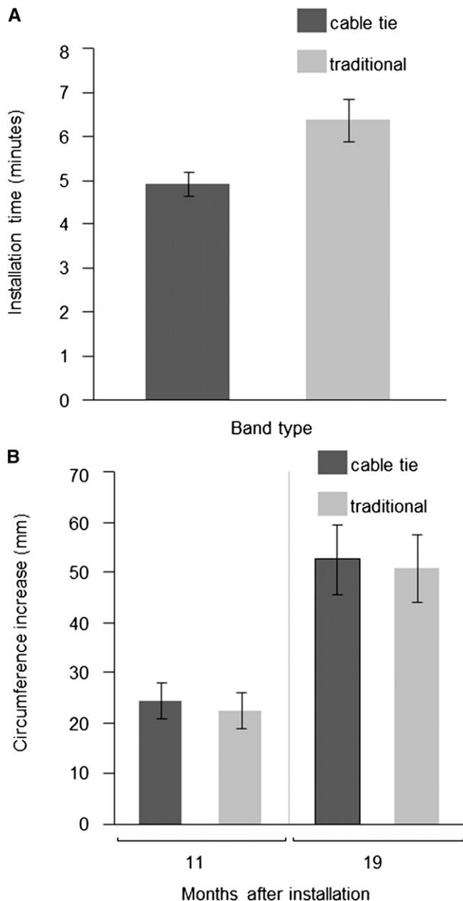
Fig. 2. (A) Time (in minutes,  $\pm$ SE) for band dendrometer installation using the traditional method vs. the modified cable tie method under ideal conditions. Tree selection and preparation times were not included in the installation times. (B) Circumference measurement (in mm,  $\pm$ SE) for traditional and modified dendrometer bands at 11 and 19 mo after band installation.
