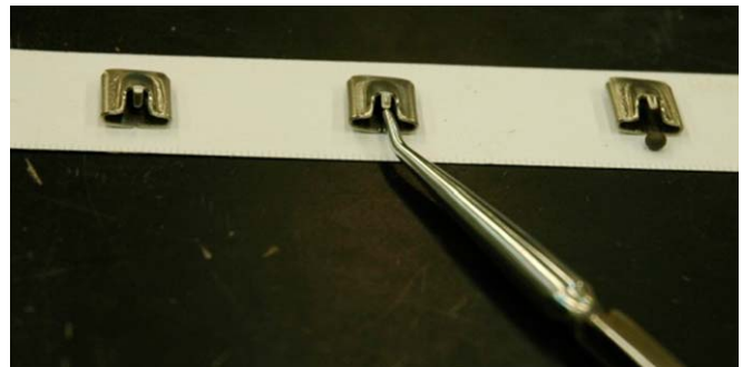
Fig. A1. Preparation of dendrometer band collar.
