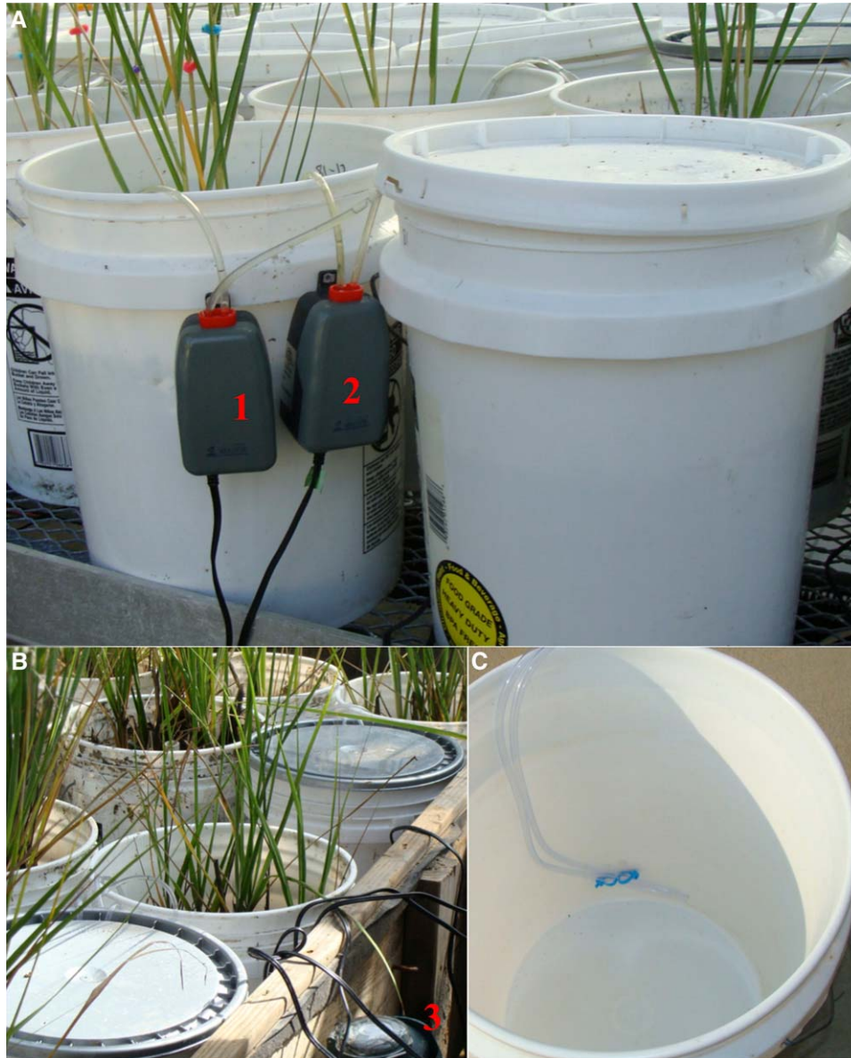
Fig. 1. Tidal simulator microcosm units consisted of one 18.9-L bucket containing a Spartina alterniflora sward connected to a second reservoir bucket (with a lid to prevent evaporation) by aquarium tubing attached to two water-lifting pumps. Pump 1 transferred water from the reservoir into the microcosm, and pump 2 transferred the water from the microcosm back into the reservoir (A). Units were connected to an outdoor timer (3) programmed to create tidal exchange every 6 h (B), and aquarium tubing extended from pumps to the bottom of both the microcosm and reservoir buckets to ensure complete transfer of water between them (C).
