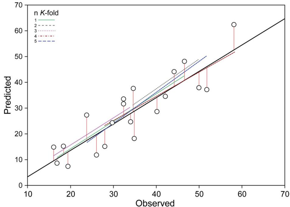
Fig. 2. Linear regression and *K*-fold cross-validation scatter plot of observed root dry weight biomass (RDW) predicted by root electrical capacitance (REC). The linear regression is  $y = 0.21x - 6.91$  ( $R^2 = 0.77$ ). Vertical red lines perpendicular to the regression line (solid black) represent the residual of the model fit, and colored lines represent *K*-fold sampling.
