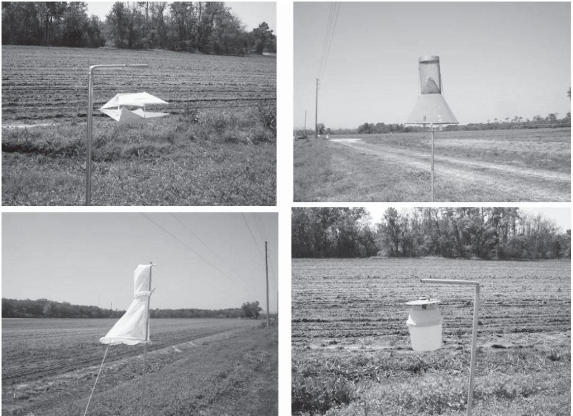
Fig. 1. Pherocon 1C (top left), wire cone (top right), Scentry Heliothis (bottom left, and Universal moth traps (bottom right).
