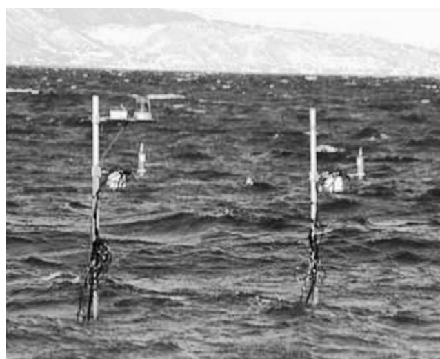
Figure 4. Ultrasonic probes used during the NOEL1 experiment to measure the directional spectrum.
