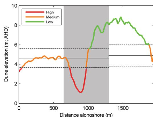
Figure 2. Comparison of 5yARI  $E_R$  with dune crest elevation at Avoca. Distance alongshore is measured south to north with the Central sector shaded. Estimated runup elevations and standard deviations are shown for each sector as solid and dashed lines respectively. Coloured lines indicate runup inundation potential.
