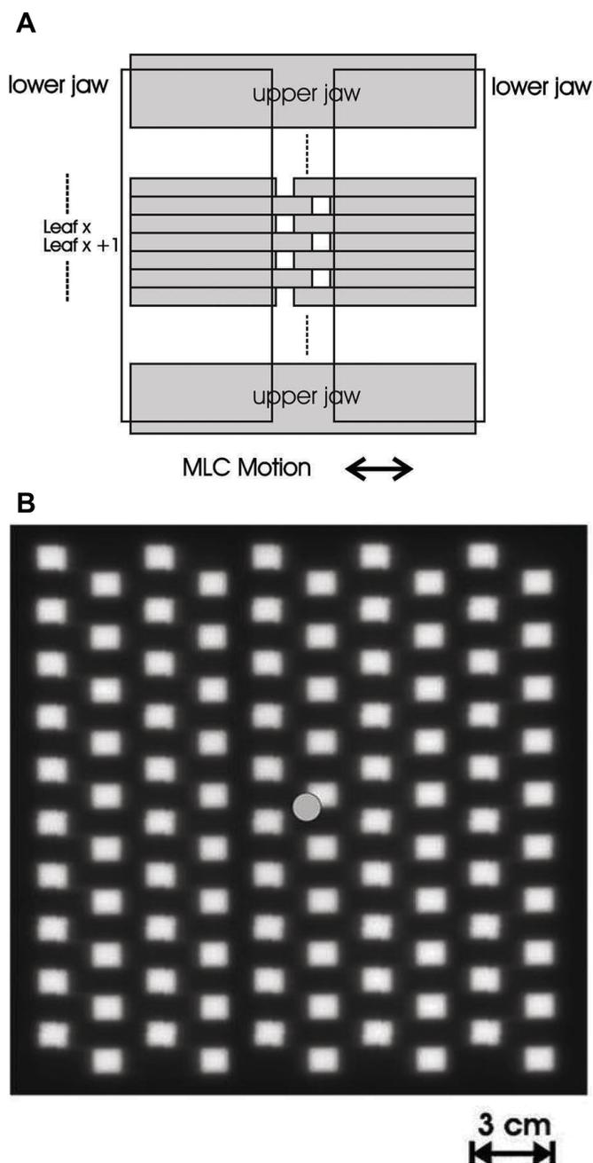
**FIG. 2.** The MLC-created GRID radiation field (4). MLCs also could be used to generate grid-like field. In this example, five separate MLC-shaped beams were used, and each defined two columns of the grid openings. The composite of the five beams gave rise to an effective “GRID” with the openings arranged in an alternating checkerboard pattern and open-to-close areal ratio of 1:3 (4).
