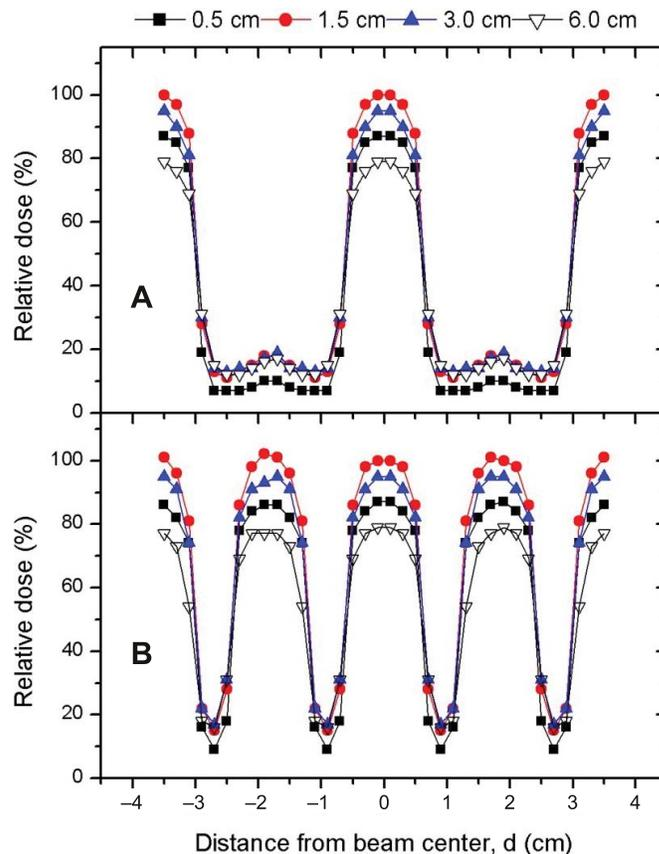
FIG. 6. Radial and transverse dose profiles of GRID therapy in a flat water phantom at 0.5, 1.5, 3.0 and 6 cm depths for a 6-MV beam. The doses were normalized to a  $10 \times 10$  cm<sup>2</sup> open field at 1.5-cm depth, and 100 cGy was applied to the open field as a standard. Panels A and B: In plane and cross plane, respectively (40).
