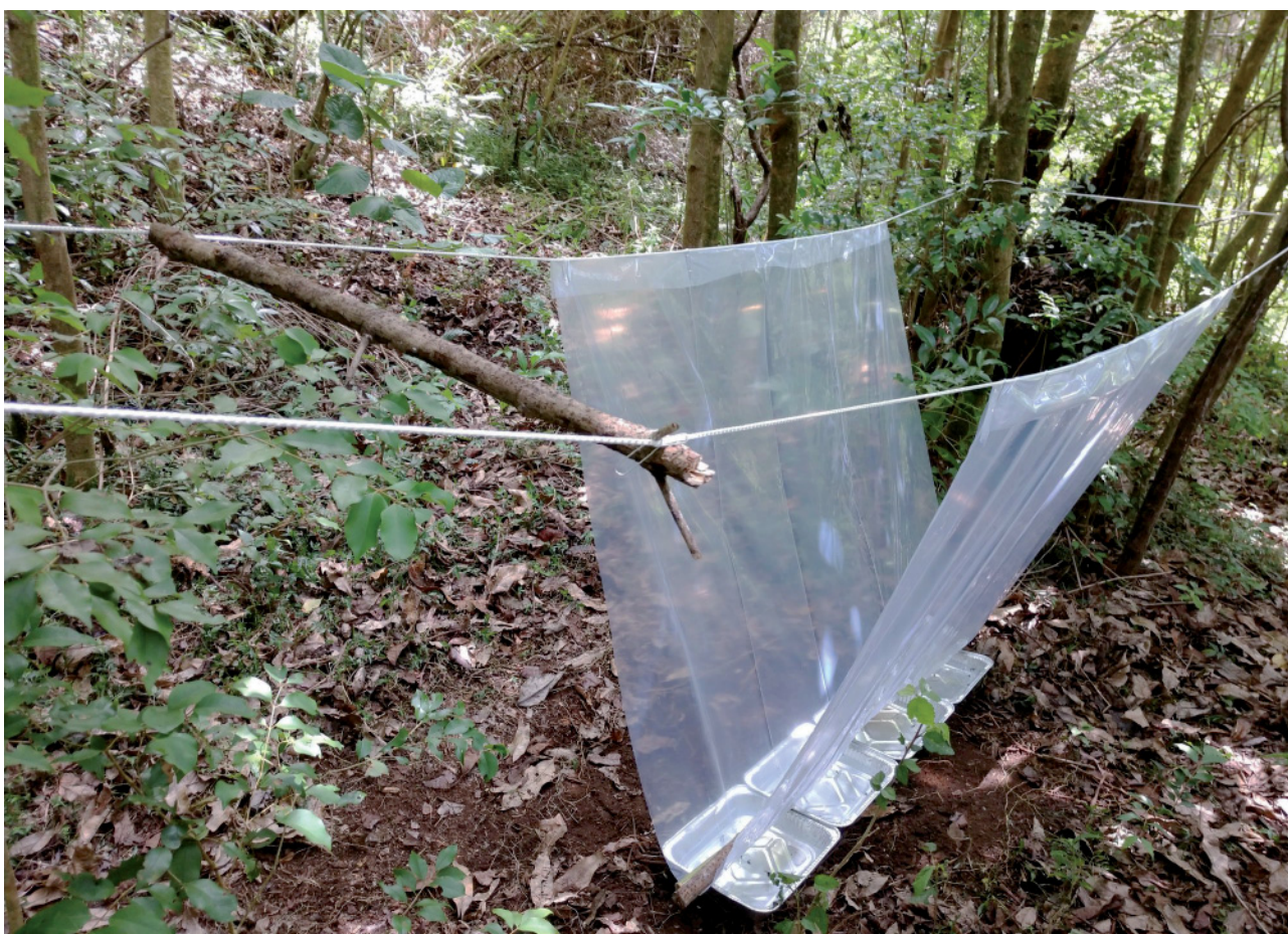
Fig. 2. Travel version of V-flight intercept trap.
