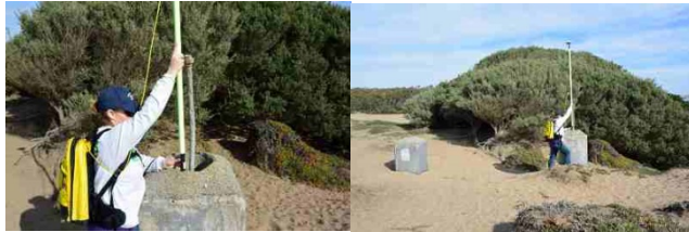
Ground Control Point 53: Peak of southern concrete pillar in former National Guard Armory.
