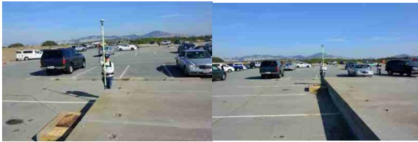
Ground Control Point 6: Northeast corner of middle concrete platform in parking lot.
