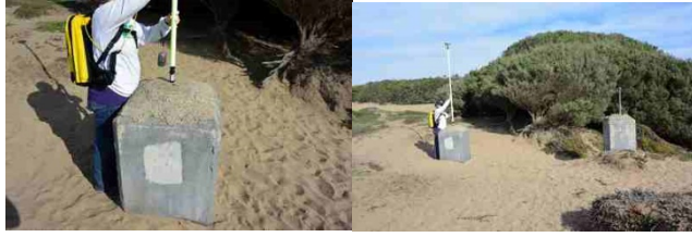
Ground Control Point 52: Peak of northern concrete pillar in former National Guard Armory.
