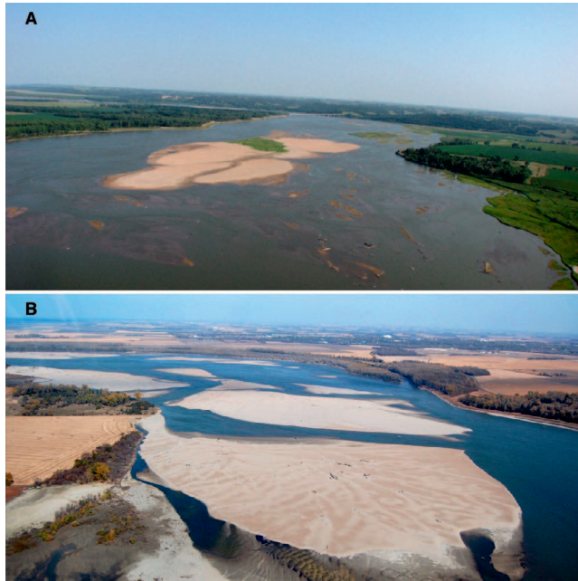
FIGURE 2. Examples of (A) pre-flood engineered sandbar habitat that was created by the U.S. Army Corps of Engineers (USACE; 2005–2009) by dredging sand from the river bottom, depositing it at the construction site, and leveling it with bulldozers (Catlin et al. 2015), and (B) post-flood natural sandbar habitat that was created through sediment deposition during the 2011 flood on the Missouri River, USA. Photos provided by the USACE.
